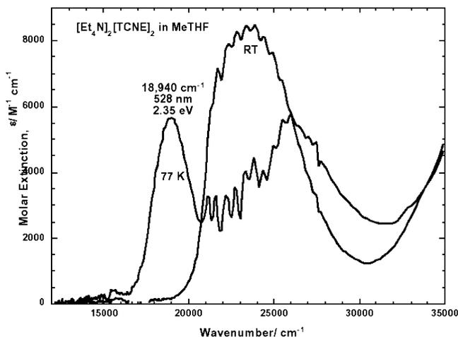
**Figure 3.** Electronic spectrum of  $(\text{TCNE})_2^{2-}$  in methyl-tetrahydrofuran at 77 K (as a glassy material) and at room temperature (RT). The absorptions shown at RT are characteristic of the  $\text{TCNE}^-$  anion (taken from ref 1b).
