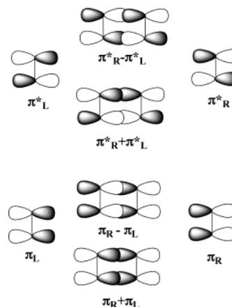
**Figure 2.** Four  $\pi$ -based four-center molecular orbitals (center) and their origins from the two left (L) and right (R) TCNE<sup>-</sup> anions' orbitals.
